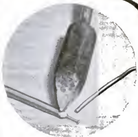
One piece of copper tubing 5" long and another longer piece are soldered to a common hose connection. The two tubes are narrowed at the end to form jets
